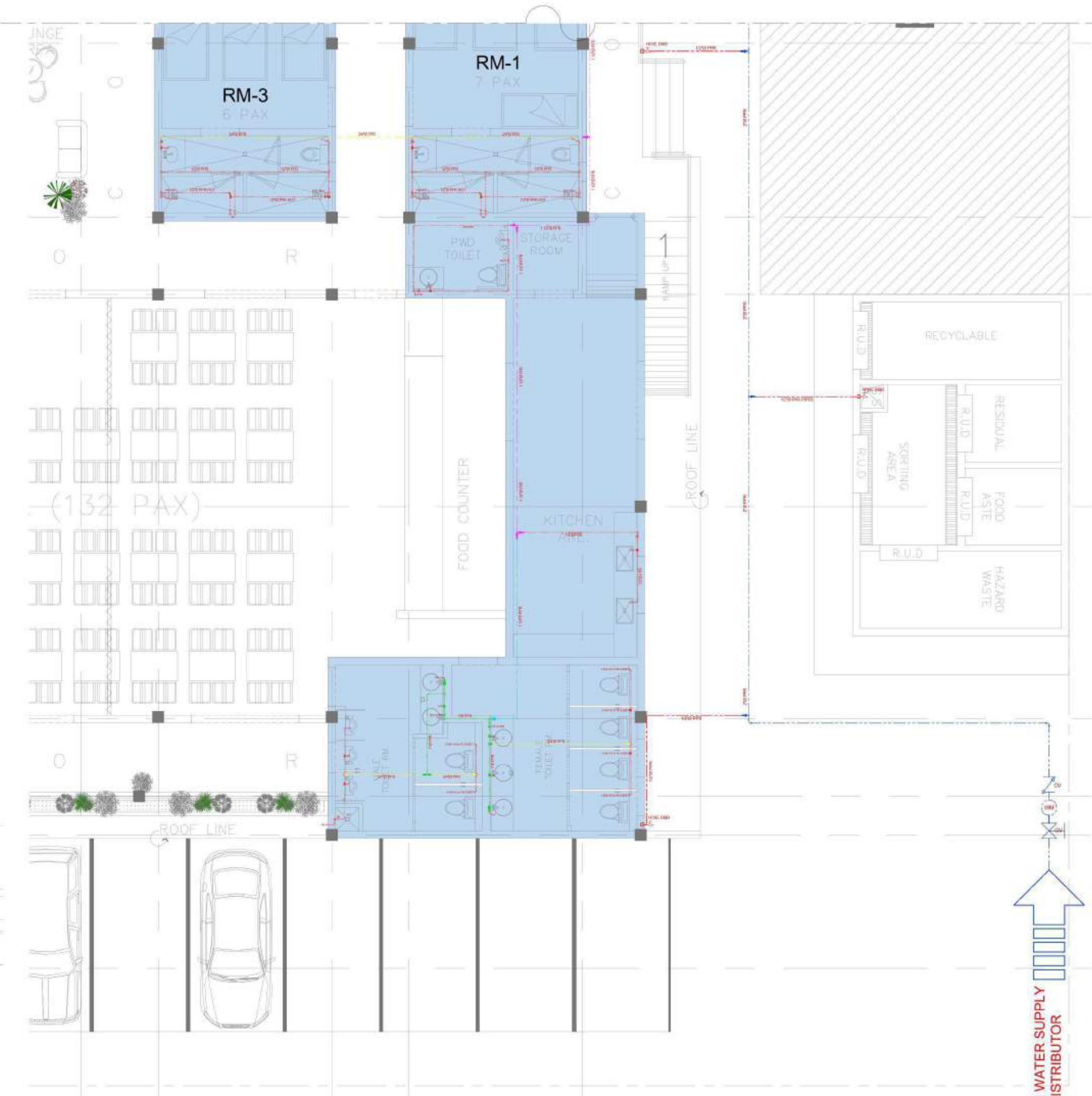
3 ZONE 1 BLOW-UP WATERLINE SYSTEM (PG-1) SCALE 1:75MTS
